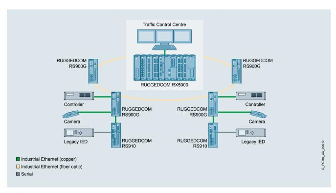
A reliable eRSTP ring network with Gigabit bandwidths can be achieved with the RUGGEDCOM RS900G.
