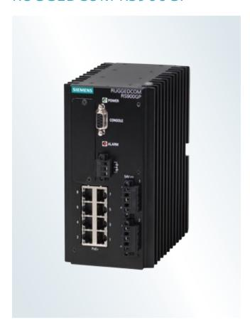
The RUGGEDCOM RS900GP is a 10-port utility-grade, fully managed Ethernet switch, providing two fiber-optic or copper Gigabit Ethernet ports and eight Fast Ethernet copper ports, each capable of supplying high power 802.3at compliant power over Ethernet.
