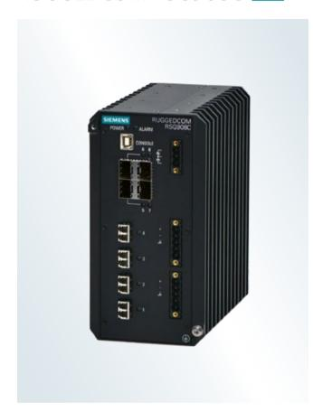
The RUGGEDCOM RSG908C is an IEEE 1588 compatible Ethernet switch, providing 4 Gigabit SFP ports and 4 Fast Ethernet fiber ports.
