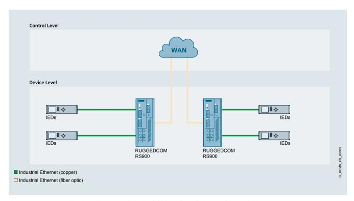
$The \ RUGGEDCOM \ RS900 \ makes it possible to \ remotely \ monitor field \ data \ using \ multiple \ types \ of \ communications.$
