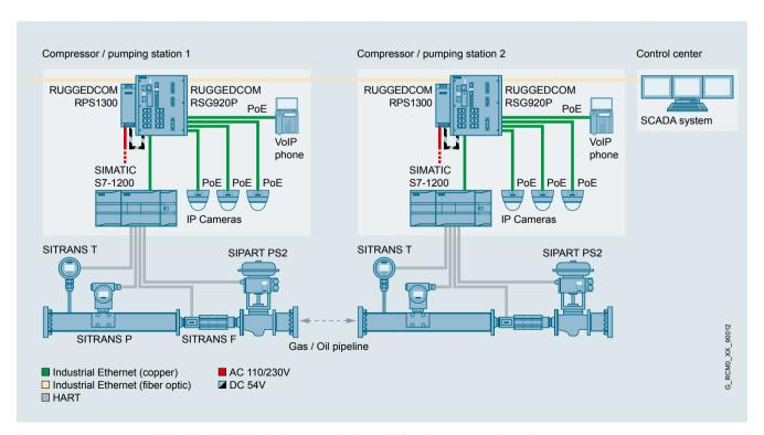
$The \ RUGGEDCOM \ RSG920P \ is \ ideal \ for \ the \ field \ level \ where \ growing \ demands \ for \ Ethernet \ connectivty \ exist.$
