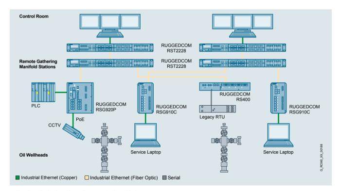
Wellhead monitoring in on shore oil  $\mbox{\sc gas}$  production with the RUGGED COM RSG910C.
