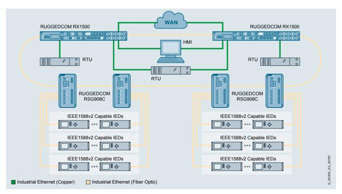
The RUGGEDCOM RSG908C allows the aggregation of large fiber optic 100BASE-FX subrings of IEDs at protection bays into 1 Gbit/s fiber optic rings while providing IEEE1588 timing.
