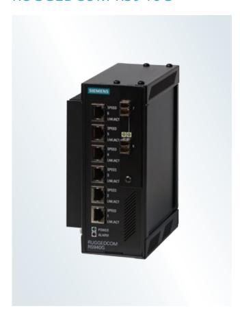
The RUGGEDCOM RS940G is a utility-grade, fully managed Ethernet switch, providing up to eight Gigabit Ethernet ports. Six 10/100/1000BASE-T triple speed copper ports are standard. An additional two Gigabit fiber or copper ports can be added.
