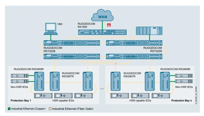
RUGGEDCOM RSG907R / RSG909R switches terminating each HSR ring can be directly connected to RSTP network via their coupling ports.
