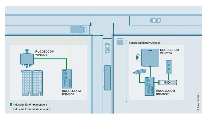
$\label{power-over-ethernet} \mbox{Multiple Power-over-Ethernet devices are powered by the RUGGEDCOM RS900GP in the field.}$
