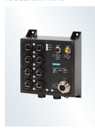
The RUGGEDCOM M969 is a MIL-STD 10-port, fully managed Ethernet switch, providing dual fiber optical Ethernet ports and eight Fast Ethernet copper ports in an IP66/IP67 rated package for protection against strong jets of water (IP66) or temporary immersion in water (IP67).
