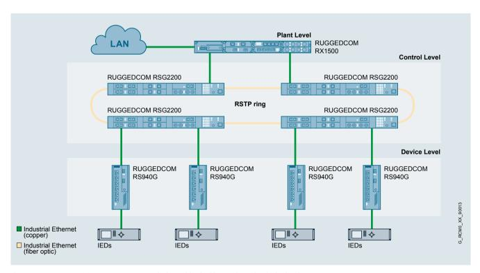
The RUGGEDCOM RS940G can connect up to 8 devices with Gigabit speeds on the device level.
