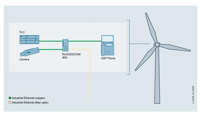
Inside the nacelle of a wind mill the RUGGEDCOM i802 enables connectivity to up to 6 Ethernet devices over copper and a backhaul over fiber-optic.
