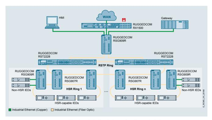
Two RUGGEDCOM RSG907R / RSG909R are used in each HSR bay ring for redundant coupling with PRP station level LANs.
