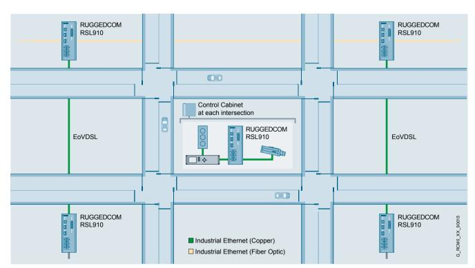
Traffic signal connectivity between intersections using a combination of existing copper cabling and fiber-optic backbone.
