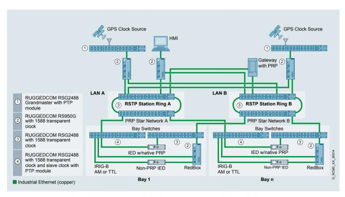
The RUGGEDCOM RS950G RedBox helps creating the most reliable redundant networks while maintaining Gigabit speeds throughout.
