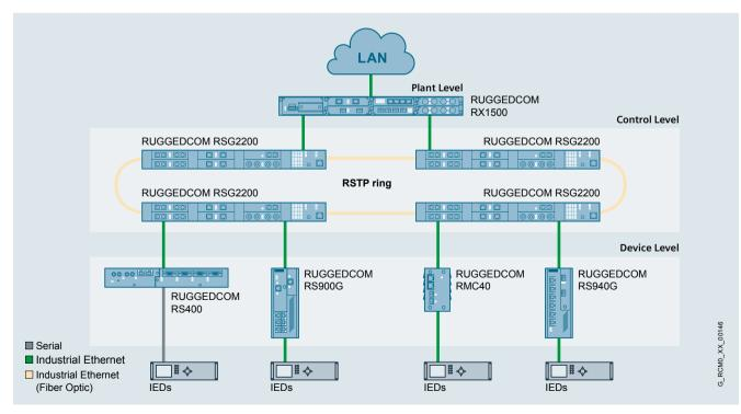
With the RUGGEDCOM RSG2200 Gigabit communication is possible for reliable and high speed connection throughout the network.
