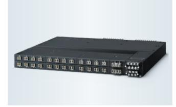
The RUGGEDCOM RSG2488 is a utility-grade, field upgradable, fully managed, 28-port Gigabit Ethernet switch with hot-swappable dual redundant power supplies. It is specifically designed to operate reliably in electrically harsh and climatically demanding environments.
