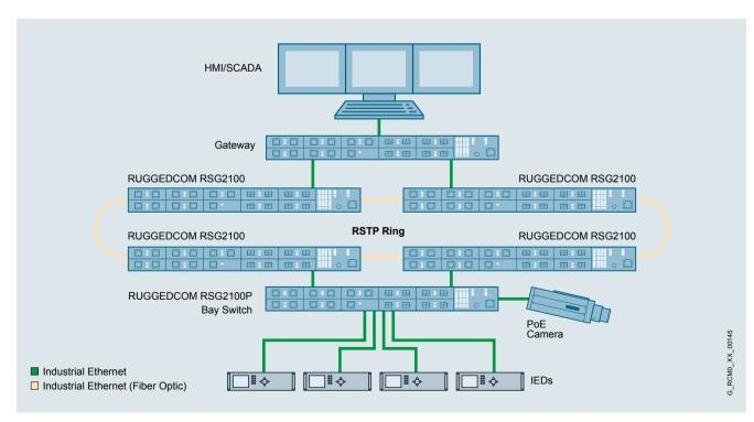
The RUGGEDCOM RSG2100 is deployed in a redundant ring based on RSTP for optimal reliability.
