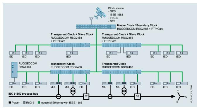
The field-modular RUGGEDCOM RSG2488 is the most versatile offering for IEEE1588 time synchronisation and can function as master, boundary, slave and transparent clock.
