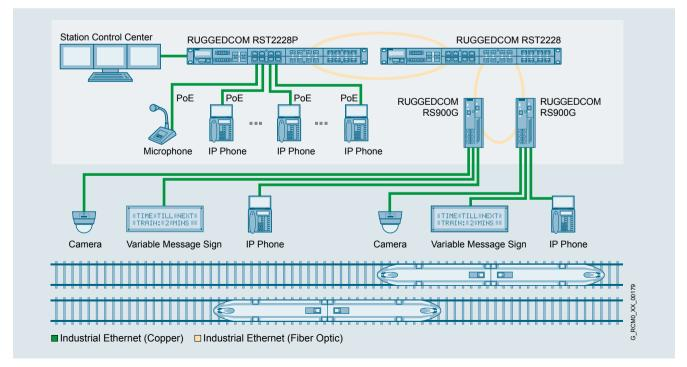
Connect a high number of Power-over-Ethernet capable VoIP-telephones and other devices to a single RUGGEDCOM RST2228P.
