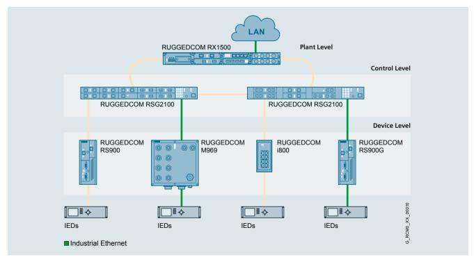
Thanks to its interface versatility the RUGGEDCOM RSG2100 is an ideal device to connect a lot of different devices using a combination of fiber optic and copper with different connector types and speeds.
