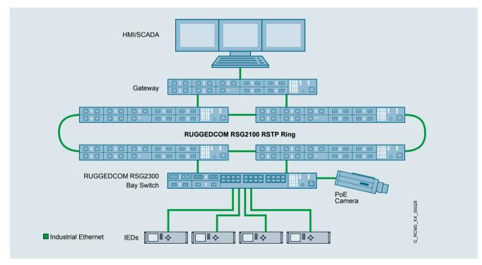
With its high port density of copper interface the RUGGEDCOM RSG2300 is ideal for connecting a large number of devices at the Bay level.
