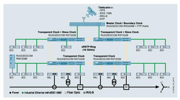
Up to 24 modern IEDs or other IEEE 1588 slaves can be connected directly to the RUGGEDCOM RST2228 via Fast Ethernet or Gigabit/s ports.
