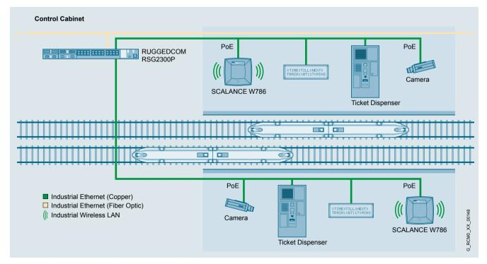
With its high number of ports the RUGGEDCOM RSG2300P is ideal for connecting Wireless LAN, cameras and other peripheral devices directly.
